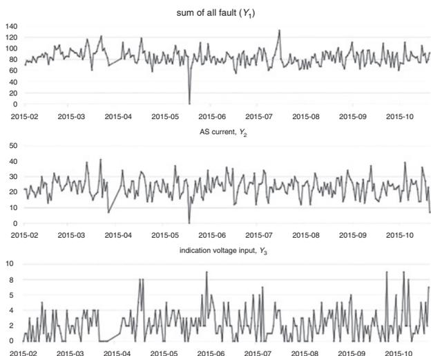
**Fig. 2** Time series plot for sum of all faults ( $Y_1$ ), fault of AS current ( $Y_2$ ) and fault of indication voltage input ( $Y_3$ ) from February to October 2015
